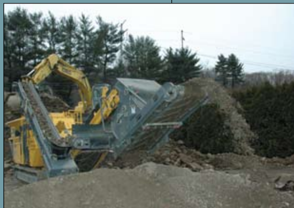
The RM80 crushes concrete, asphalt and rock into a 3/4-inch product.
